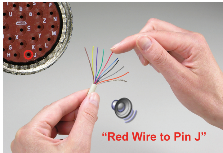
Figure 7 - Electrical sensing of unattached wires greatly increases assembly speed.
